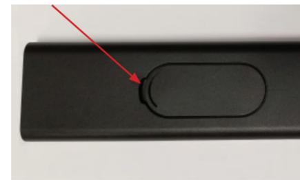
Install the CR2032 with the positive (+) side facing up in the slot sliding the battery under the small lip by the "+" symbol.
