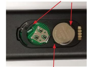
To remove battery, lift by inserting a small object in the small gap opposite the lip, and pry upwards. Dispose of the battery in accordance with the local regulations for lithium battery disposal.
